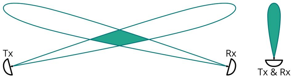
Figure 1. The directional antenna beams of a bistatic (left) and a monostatic (right) radar, with the detection region show (filled region).
