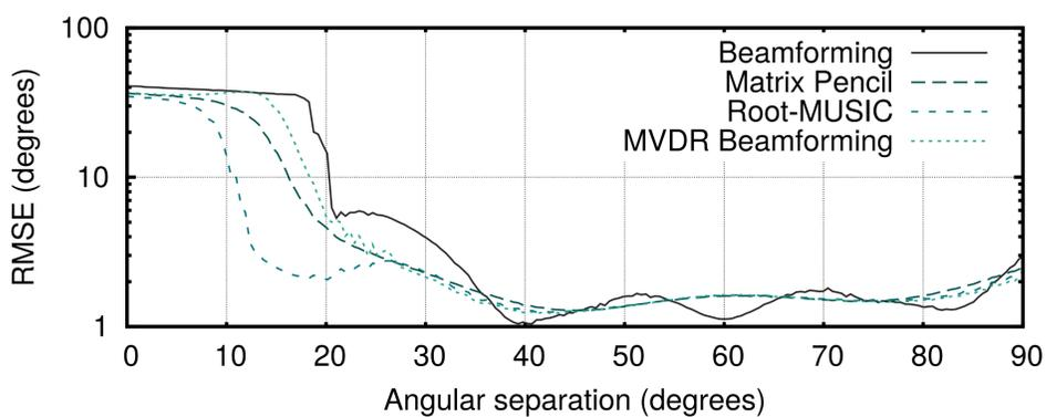
Figure 3. Broadside accuracy of a five-element linear array with two signals.
