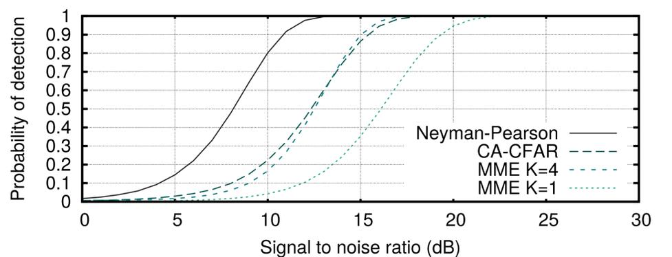
Figure 4. Probability of detection for a five element array with  $PFA=10^{-3}$ .
