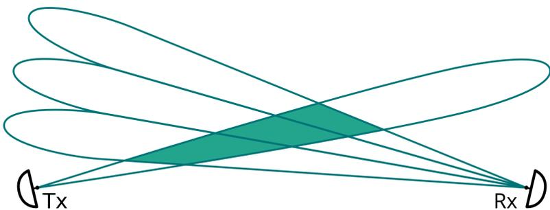
Figure 2. Fan-beam bistatic configuration, with detection region (filled).
