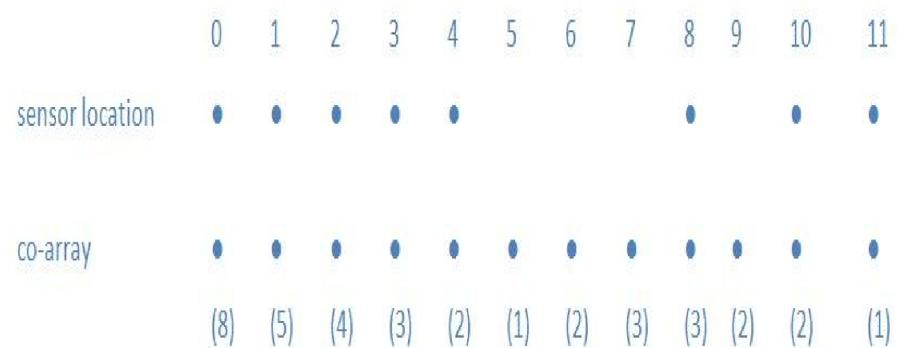
**Figure 1.** Example array geometry where the array geometry is a combination of uniform linear array and a nonuniform linear array. This is the Partly Filled Nonuniform Linear Array (PFNLA)
