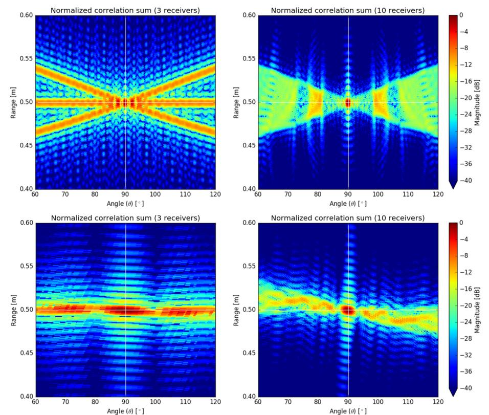
Figure 2. Simulated return form an ideal point target placed at a range of 0.5 m with  $\theta = 90^\circ$ . The top two results are obtained using a linearly-spaced array of receivers, and the bottom two using an array generated by using the process described in [3].
