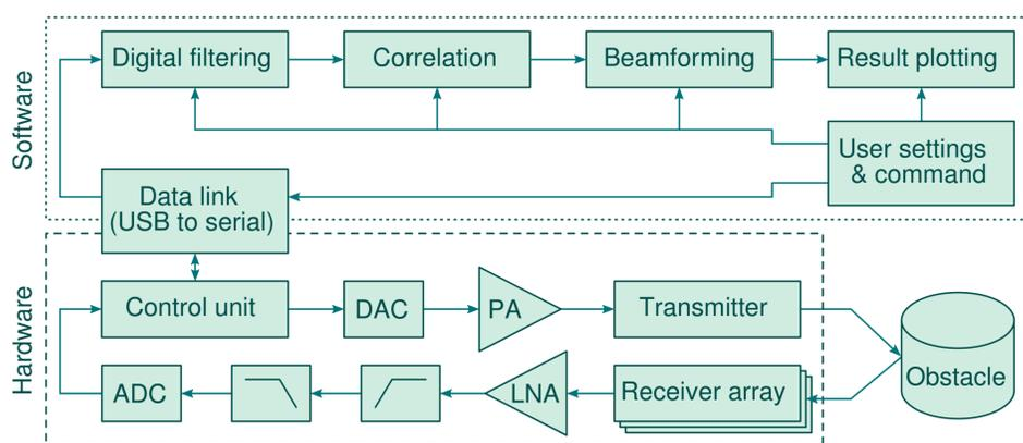
Figure 1. High-level functional block diagram of the complete system.
