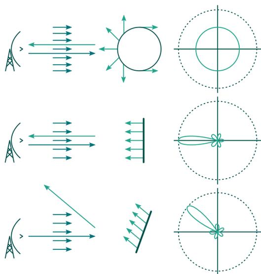
**Figure 1.** Effect of directivity on backscatter from objects with different shapes and orientations and the relative magnitude of backscatter of these shapes. [1].
