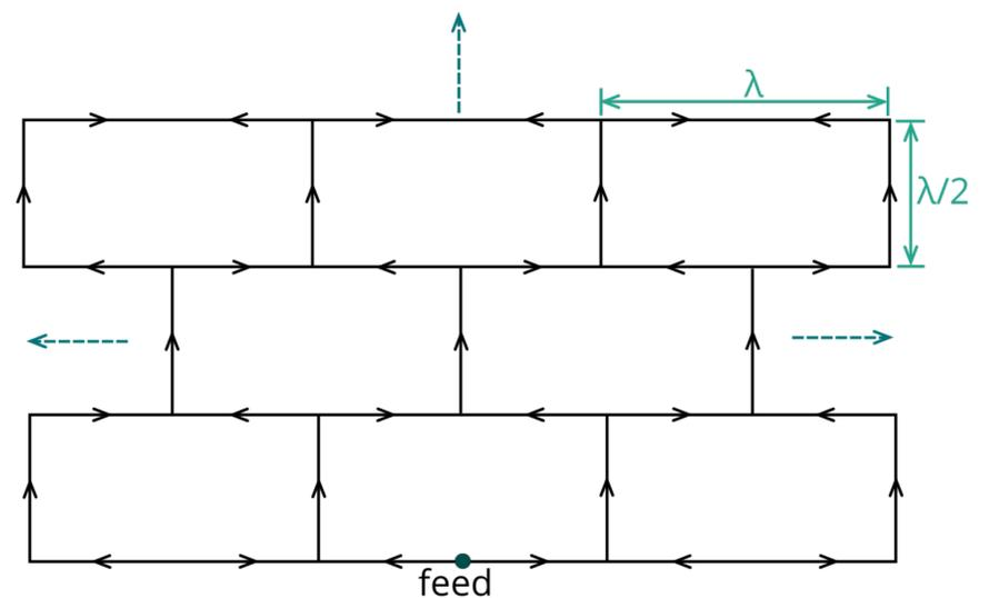
**Figure 2.** The basic brick wall antenna.
