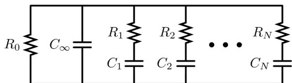
Figure 1. RC network model of the characteristics of the earth as a conductor.
