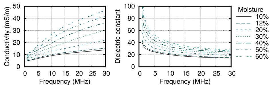
Figure 2. Calculated conductivity and dielectric constant curves for various soil moisture percentages.
